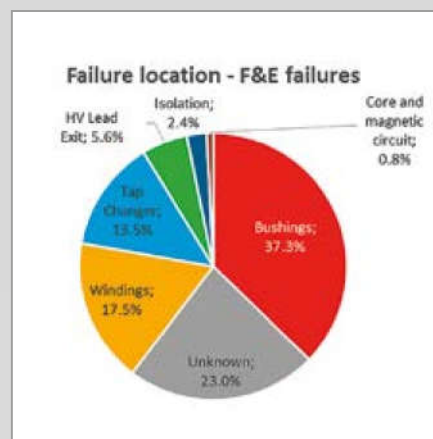
Figure 1. Failure locations of fires and explosions of power transformer failures (left) and external effects of bushing failures (right) [1]
