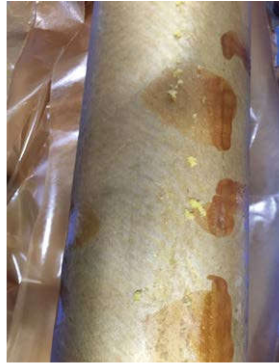
Figure 6. X-wax found on the most-inner layer of the EHV bushing disected
