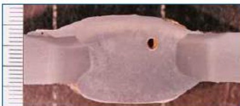
Slika 15. Makroizbrusak vrata tračnice uzorka 5 Figure 15. Macrosection of rail neck weld on sample 5
