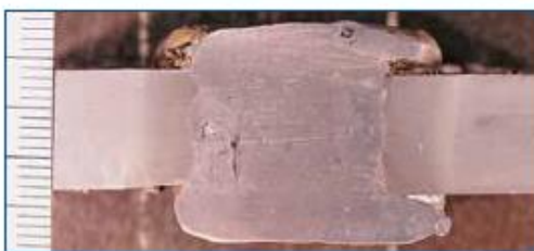
Slika 14. Makroizbrusak vrata tračnice uzorka 3 Figure 14. Macrosection of rail neck weld on sample 3
