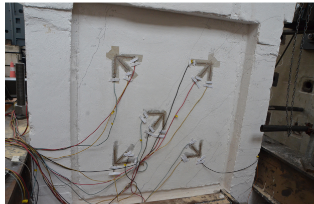
(a) Cracking pattern
