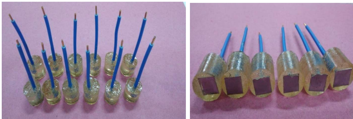
Figure 2. Specimen 304SS used as working electrode
