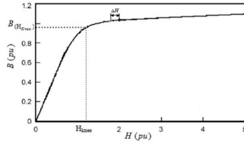
Fig. 3. Typical B-H curve of a magnetic core
