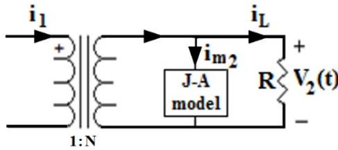
Fig. 2. The current transformer model [14]
