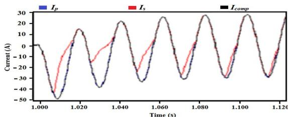
(b) Primary ( $I_p$ ), secondary ( $I_s$ ) and compensated ( $I_{comp}$ ) currents for proposed method
