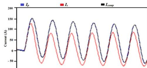
(b) Primary ( $I_p$ ), secondary ( $I_s$ ) and compensated ( $I_{comp}$ ) currents for proposed method
