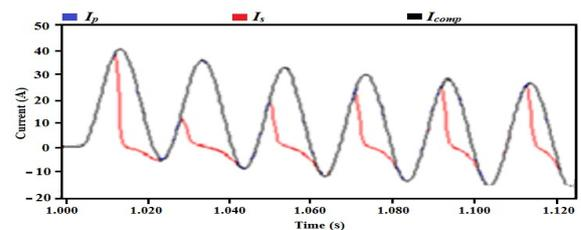
(b) Primary ( $I_p$ ), secondary ( $I_s$ ) and compensated ( $I_{comp}$ ) currents for proposed method
