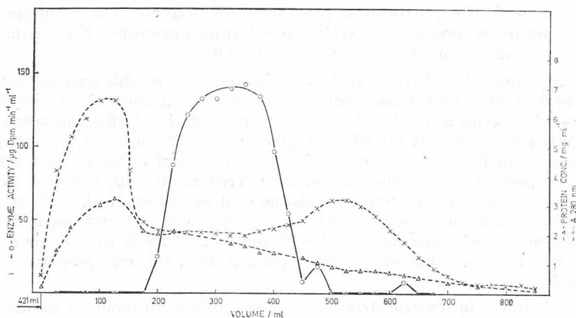
Figure 1. Gel filtration of 1.2 g of Dpm decarboxylase active ammonium sulphate precipitate, on  $5 \times 84$  cm column of Sephadex G-150 in 0.01 M Na-phosphate buffer, pH 6.8, containing 0.1 mM BAL and PyrP. Flow rate was 48 ml/h, and each fraction contained 12 ml. Protein concentration was determined according to Lowry et al.<sup>14</sup>
