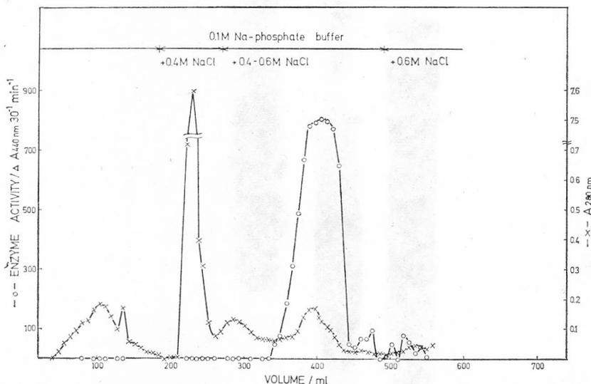
Figure 3. Chromatography of 107 mg of Dpm decarboxylase active fraction from hydroxylapatite column on  $1.5 \times 25$  cm column of DEAE-Sephadex A-50 equilibrated in 0.1 M Na-phosphate buffer, pH 6.8, containing 1 mM 2-ME and 0.1 mM PyrP. Elution was performed as indicated with a combination of stepwise and linear NaCl gradients, composed of equal volumes of 0.4 and 0.6 M NaCl in the same buffer. Flow rate was 12 ml/h and fractions of 4 ml were collected.
