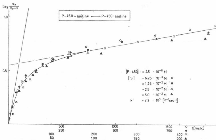
Figure 2. Aniline binding reaction to the oxidized cytochrome P450. pH 7.4,  $T = 22^\circ\text{C}$ , phosphate buffer.  $[P450] = 2.5 \cdot 10^{-6} \text{ M}$ ,  $[S] = 6.25 \cdot 10^{-3} \text{ M}$  (○),  $1.25 \cdot 10^{-2} \text{ M}$  (◻),  $2.5 \cdot 10^{-2} \text{ M}$  (△),  $5.0 \cdot 10^{-2} \text{ M}$  (▲).  $x$ ,  $x(e)$  cf. Figure 1.
