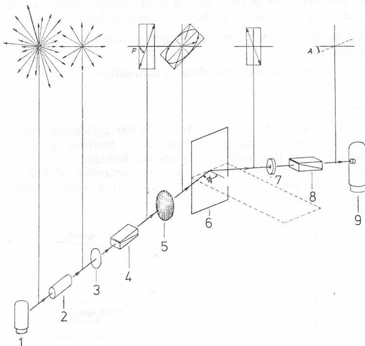
Figure 1. Schematic arrangement of the ellipsometer: light source (1), filter (2), collective lenses (3), polarizer (4), compensator (5), reflecting and adsorbing surface (6), aperture (7), analysator (8), phototube (9).
