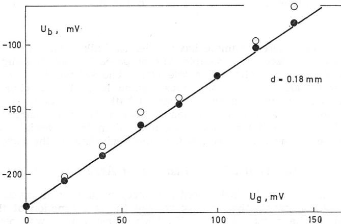
Fig. 4 — Bucking voltage  $U_b$  as a function of support voltage  $U_g$ . Performed with  $\text{SiO}_2$  sample.  $d$  — distance between sample and electrode. Blank points — first response; black points — results obtained after 5–10 minutes.
