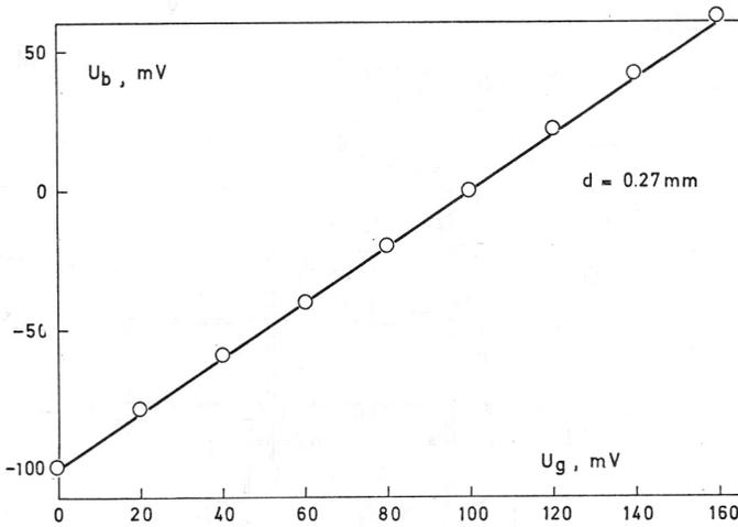
Fig. 3 — Bucking voltage  $U_b$  as a function of applied support voltage  $U_g$ .  $d$  — distance between sample and vibrating electrode. Performed with stainless steel sample.
