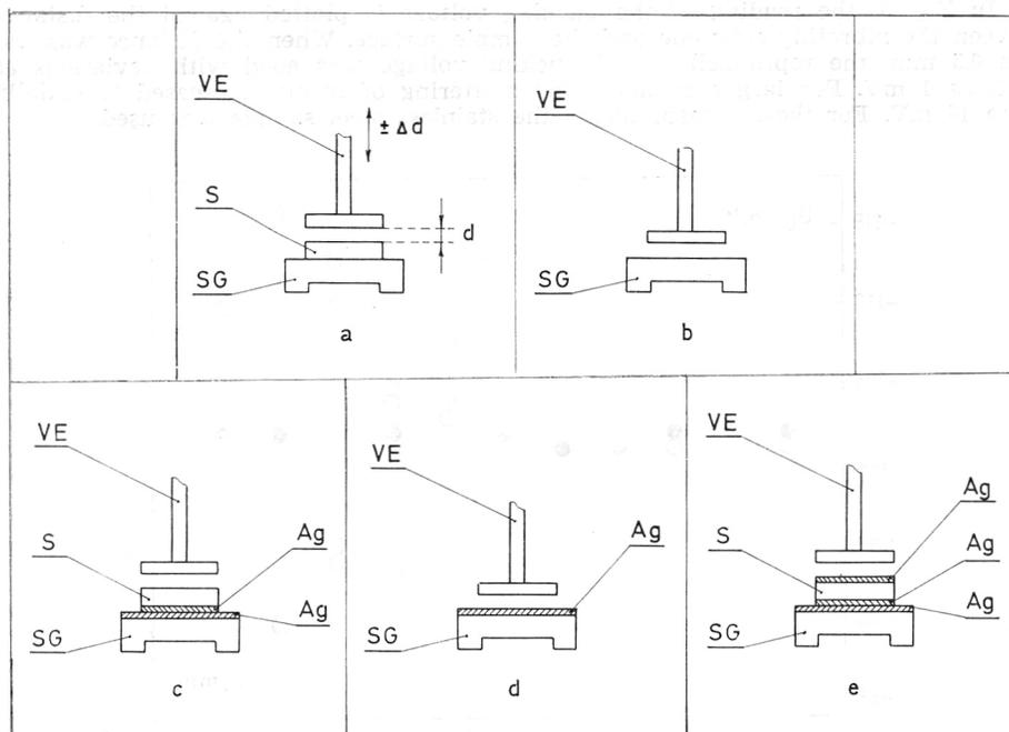
Fig. 6 — The positions of vibrating electrode against the sample and its support. SG — support; S — sample; VE — vibrating electrode; Ag — silver coating.
