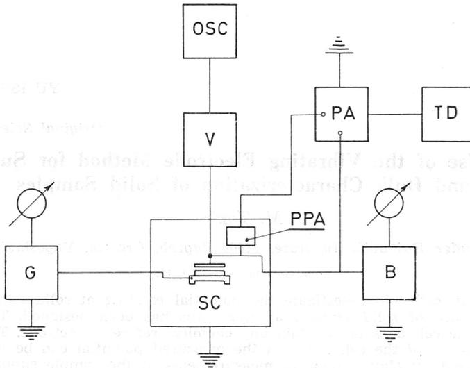
Fig. 1 — Block schematic diagram. G — potential divider for supplying the sample support; B — potential divider, the source of bucking voltage; SC — sample cell; OSC — RC oscillator, 200 Hz; V — mechanic vibrator; PPA — input stage of preamplifier; PA — preamplifier; TD — 1232 — A General Radio tuned amplifier and detector
