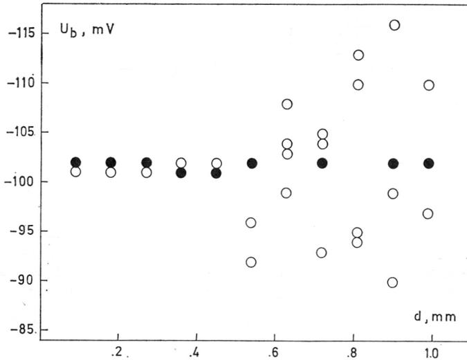
Fig. 5 — Bucking voltage against distance between sample surface and electrode  $d$ . Performed with stainless steel sample.
