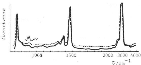
Fig. 6. I.r. spectrum of polyethylene degradation products in the presence of cyclopentadiene,  $T = 350^{\circ}\text{C}$ , exposure for 1 hr; (—) before; (---) after degradation.
