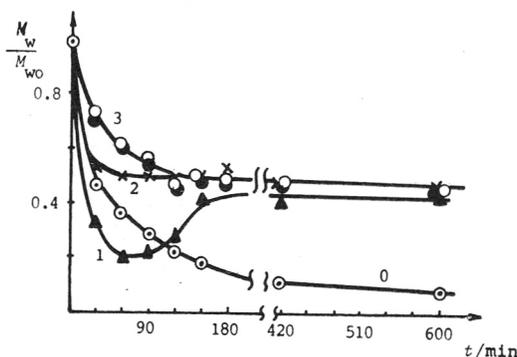
Fig. 1. The kinetic of thermal degradation of low-density polyethylene in the presence of difference inhibitors (gravimetric).  $T = 350^\circ\text{C}$ . Curves: 0—without inhibitor; 1—0.5% by wt. *p*-FcAn; 2—0.5% by wt. Fc; 3—0.3% cyclopentadiene (CPD,  $\circ$ ); —0.3% cyclohexadiene (CHD,  $\bullet$ ).
