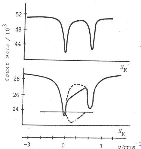
Fig. 5.  $\gamma$ -resonance spectrum of  $p$ -FcAn in polyethylene under different conditions of thermal treatment:
