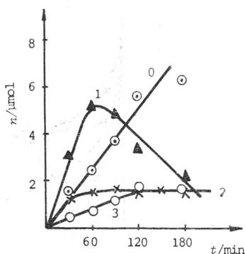
Fig. 4. The kinetics of the chain cleavage of polyethylene macromolecules on thermal degradation in the presence of various additives.  $n$  — number of chain scissions in polymer sample ( $1.4 \cdot 10^{-3}$  mol  $C_2H_4$ ).  $T = 350^\circ C$ . Curves: 0 — without inhibitor; 1 — 0.5% by wt.  $p$ -FcAn; 2 — 0.5% by wt. Fc; 3 — 0.3% by wt. CPD.
