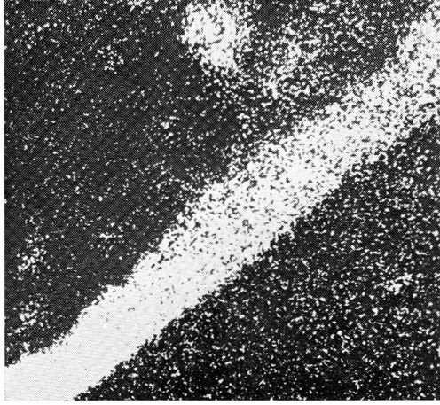
Fig. 7. A characteristic X-ray picture ( SK - \alpha ) obtained on the diffusion couple U - US_2 .
