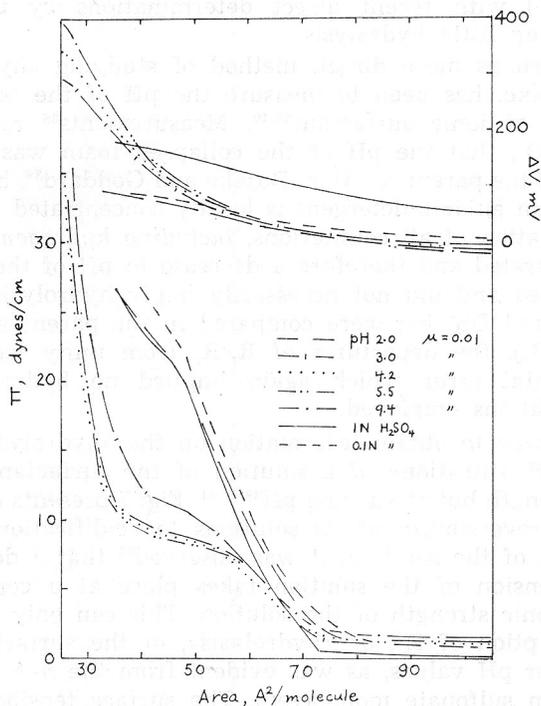
Fig. 6. Effect of pH on  $\pi$ -A and  $\Delta V$ -A isotherms of nonadecylbenzene sulfonate at 25 °C. Substitutions are 0.01 ionic strength (NaOH of HCl/NaCl) except for 0.1 N H<sub>2</sub>SO<sub>4</sub> and 1 N H<sub>2</sub>SO<sub>4</sub>.
