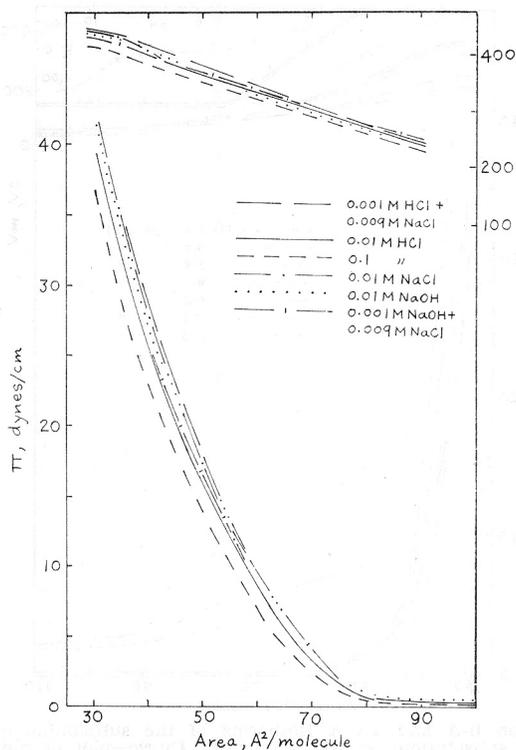
Fig. 8. Effect of pH on the  $\pi$ -A and  $\Delta V$ -A isotherms of the sulfobetaine at 25° C. Substitutions are of 0.01 ionic strength except for the 0.1 M HCl.
