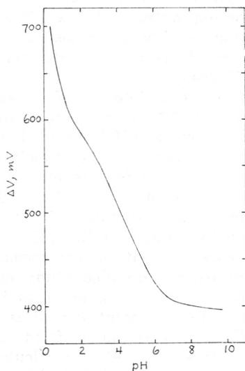
Fig. 5. Variation with pH of  $\Delta V$  for close packed films of dioctadecyl phosphate on subsolutions of ionic strength 4, at 20° C.
