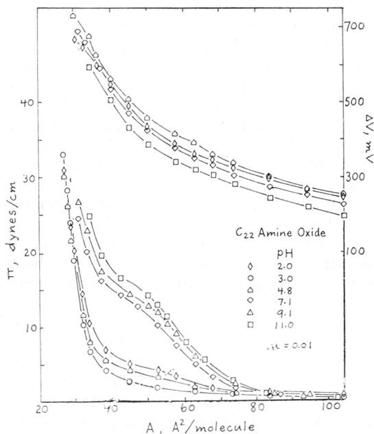
Fig. 3. Effect of pH on  $\pi$ -A and  $\Delta V$ -A of docosyldimethylamine oxide at 25° C. Subsolutions are of 0.01 ionic strength (NaOH or HCl/NaCl).
