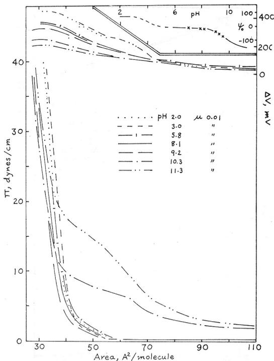
Fig. 9. Effect of pH on  $\pi$ -A and  $\Delta V$ -A isotherms of the sulfoamine on 0.01 ionic strength (NaCl + HCl or NaOH) subsolutions at 25° C. Inset: Curve-plot of measured values of  $\Delta V$  ( $40 \text{ \AA}^2$ ) vs. pH; x — calculated values of  $\psi_0$  ( $40 \text{ \AA}^2$ ) vs. pH.
