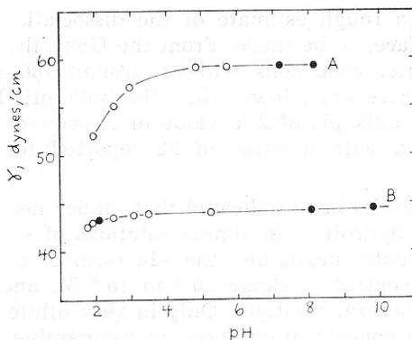
Fig. 7. Surface tension vs. pH for  $10^{-3}$  M sodium dodecane sulfonate at  $25^{\circ}$  C. Curve A,  $10^{-2}$  ionic strength; curve B,  $10^{-1}$  (●, solutions taken to lowest pH followed by NaOH addition).
