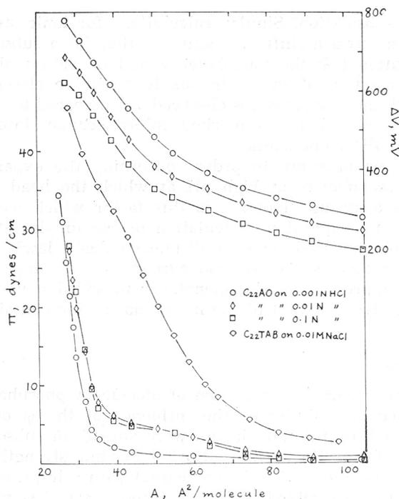
Fig. 4. Effect of HCl concentration on  $\pi$ -A and  $\Delta V$ -A isotherms of docosyldimethylamine oxide at 25° C. Isotherm ( $\pi$ -A) for docosyltrimethylammonium ion included.
