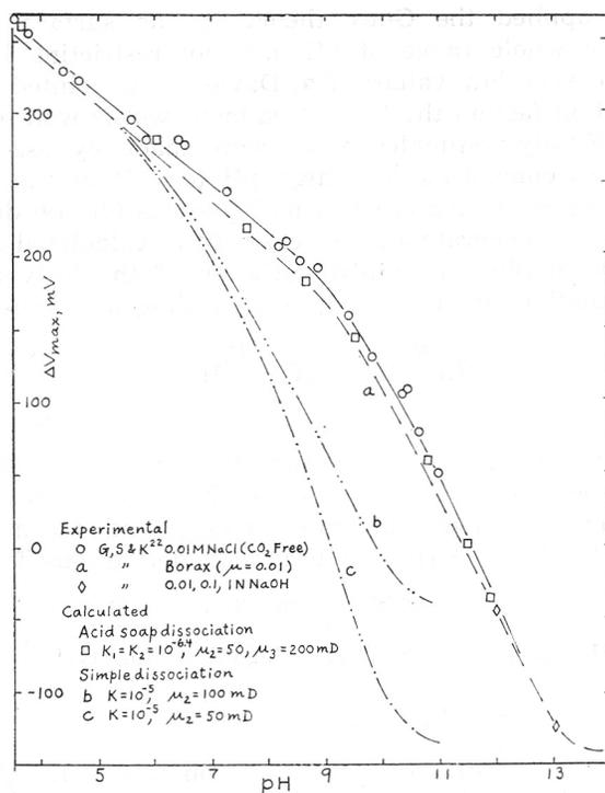
Fig. 2. Experimental  $\Delta V_{\max}$ -pH curves for behenic acid monolayers on 0.01 ionic strength solutions at 26 °C; points for 0.1 and 1.0 M NaOH included. Calculations are for  $c = 0.01$  M.
