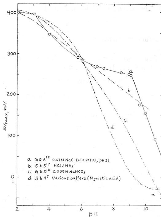
Fig. 1. Variation with pH of  $\Delta V_{\max}$  for close packed films of stearic (and myristic) acid reported by various workers.
