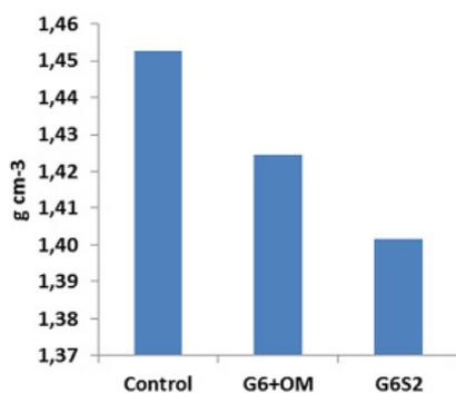
**Figure 2.** Amendment effect on bulk density
