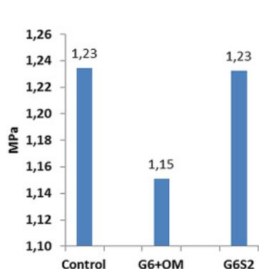
Figure 4. Amendment effect on penetration resistance
