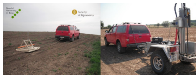
Figure 1. Measurement of soil EC by CMD-6L device (left) and soil sampling with Duoprob 60 device
