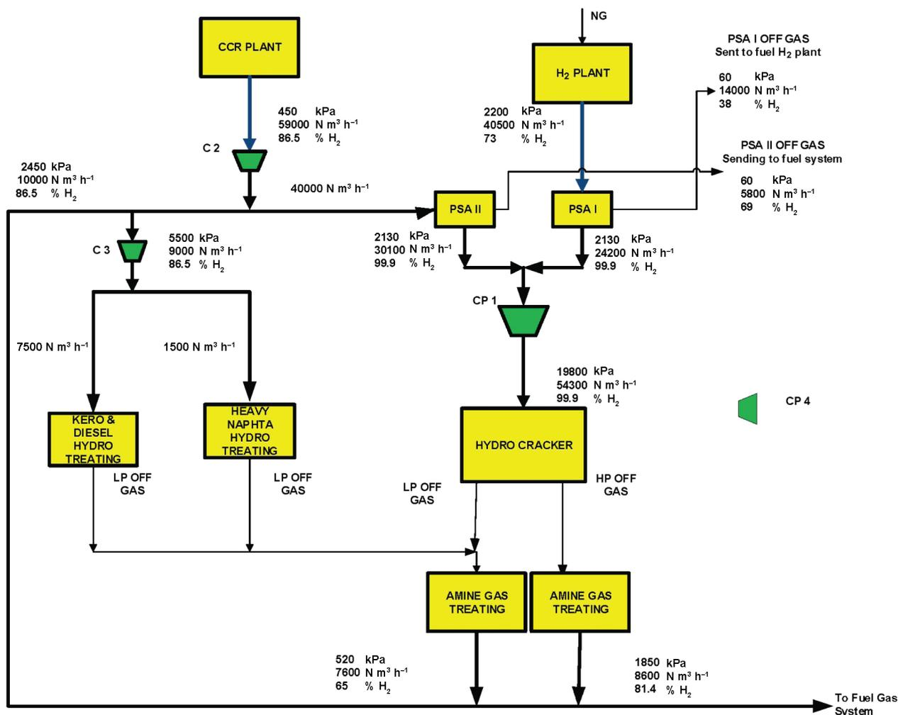
Fig. 2 – Existing refinery hydrogen network<sup>27</sup>
