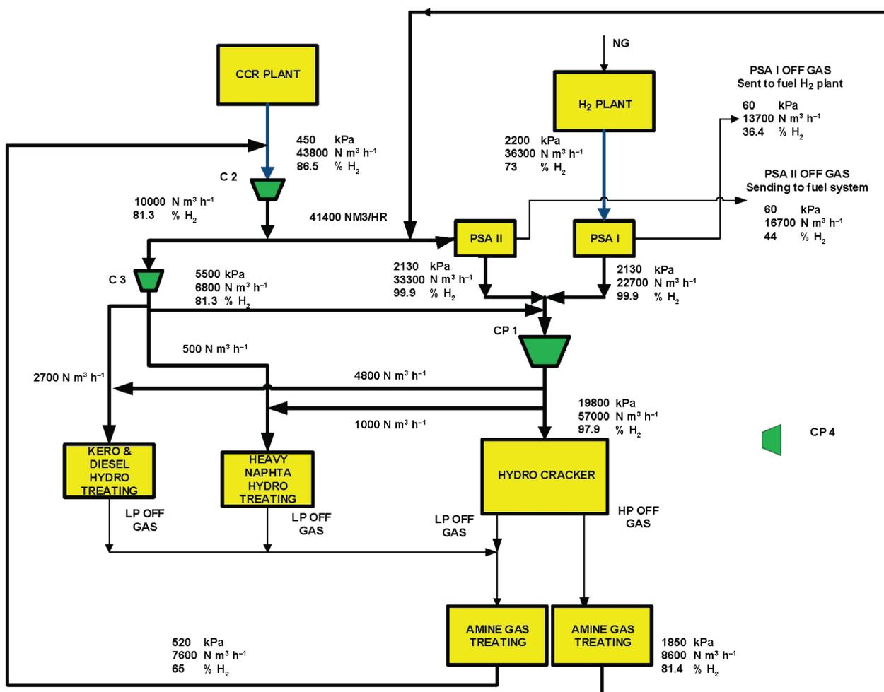
Fig. 3 – Optimum network design for Case 1
