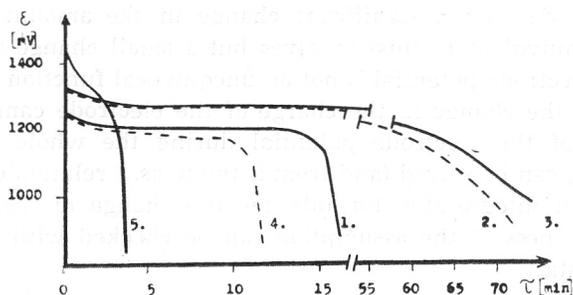
Fig. 2. Oxidation of various compounds by NiOOH electrode in N KOH solution on a Pt-sheet of 10 cm<sup>2</sup> surface area.
