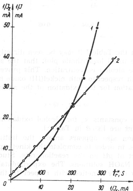
Fig. 4. Oxidation of 0.1 M ethanol on a NiOOH electrode.
