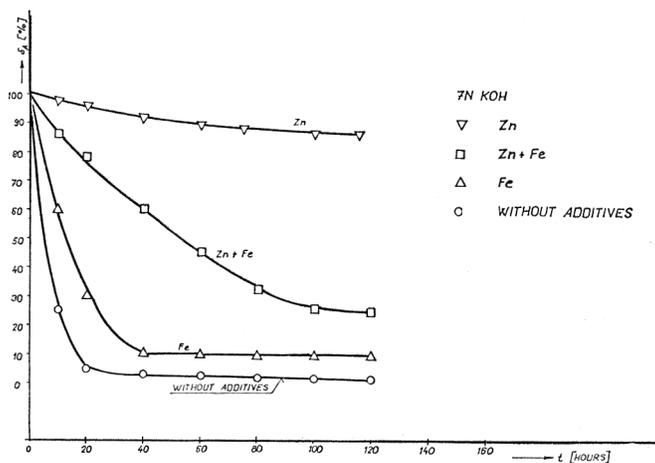
Fig. 7. Limiting of Zn effect upon drop of oxygen electrode activity in unloaded condition without oxygen pressure by action of Fe.
