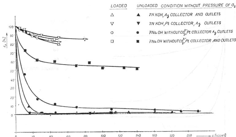
Fig. 4. Effect of various materials of collector construction upon drop of  $\text{O}_2$  electrode activity
