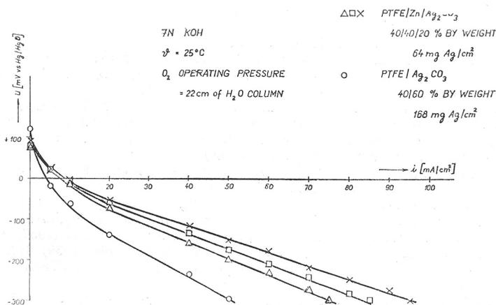
Fig. 11. Polarisation curves of oxygen electrodes on the base of PTFE | Zn | Ag and PTFE—Ag.
