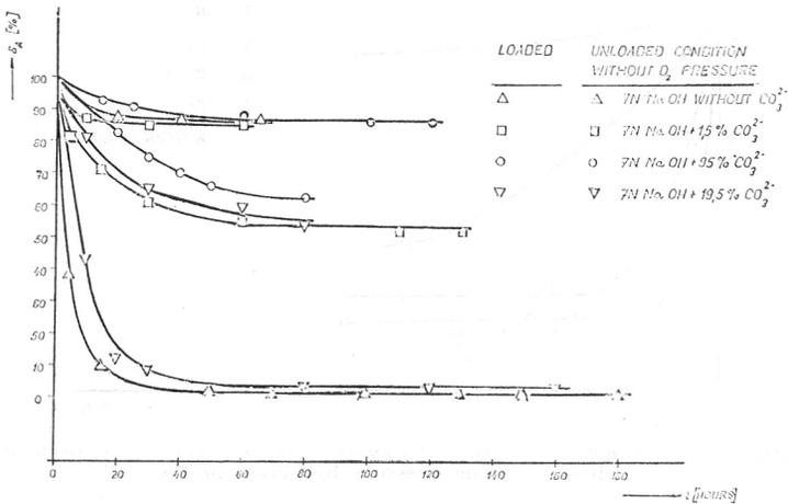
Fig. 9. Effect of  $CO_3^{2-}$  upon oxygen electrode activity.
