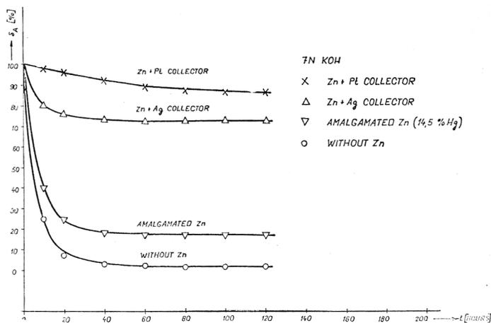
Fig. 6. Effect of Zn upon drop of oxygen electrode activity in unloaded condition without oxygen pressure.
