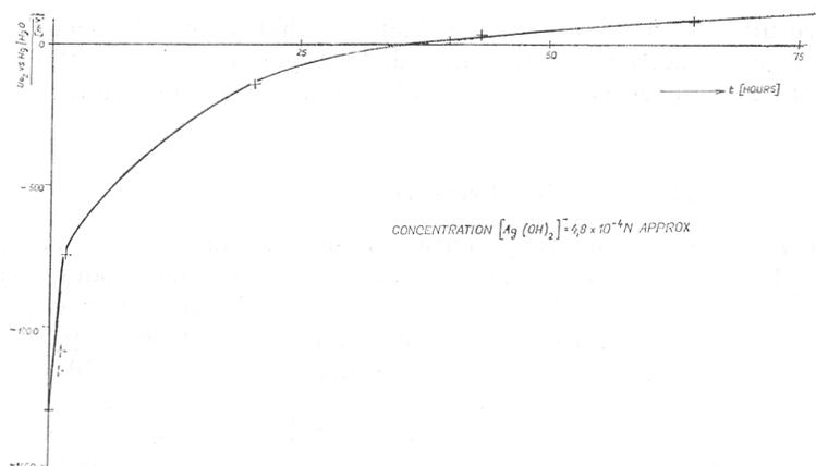
Fig. 10. Change of Zn-PTFE electrode system potential effected by  $\text{Ag}^{\text{I}}$  present in 7 N KOH in form of  $[\text{Ag}(\text{OH})_2]^-$ .
