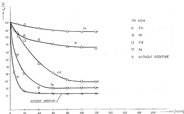
Fig. 5. Effect of Zn, Ni, Cd, and Fe upon drop of oxygen electrode activity in unloaded condition without pressure of  $O_2$ .
