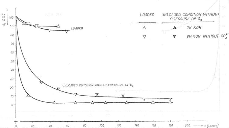
Fig. 1. Drop of oxygen electrode activity when loaded and in unloaded condition without pressure of O<sub>2</sub>.
