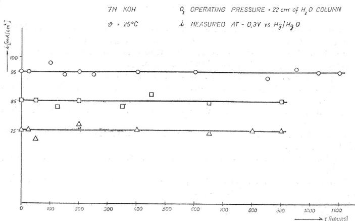
Fig. 12. Time dependence of current density of oxygen electrodes on the base of PTFE | Zn | Ag<sub>2</sub>CO<sub>3</sub> (40 : 40 : 20% by weight, 64 mg Ag/cm<sup>2</sup>).
