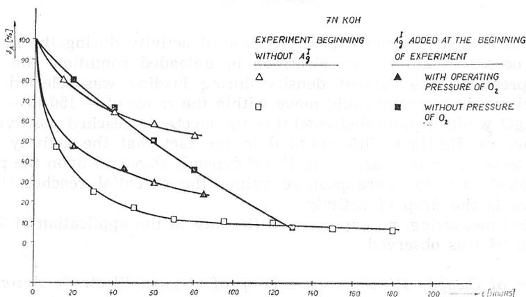
Fig. 3. Effect of Ag<sup>I</sup> added into electrolyte at the beginning of experiment, upon drop of O<sub>2</sub> electrode activity without loading.
