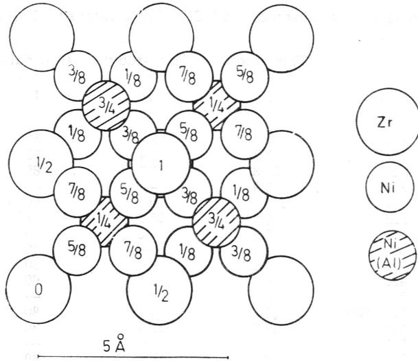
Fig. 2. The projection of the unit cell of  $ZrNi_4(Ni,Al)$ .
