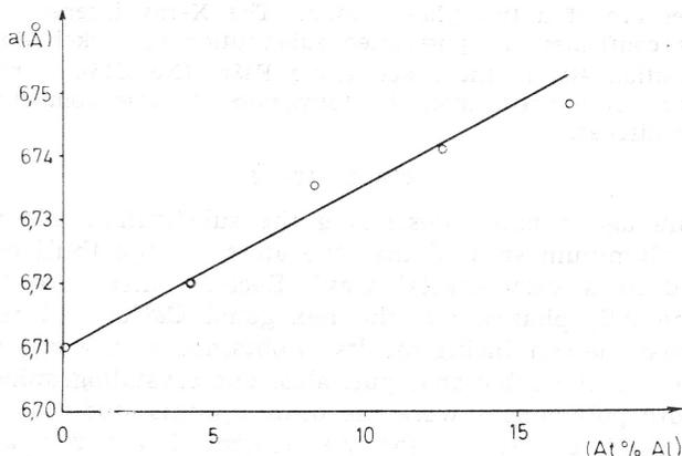
Fig. 1. The lattice parameter variation in the single phase region.
