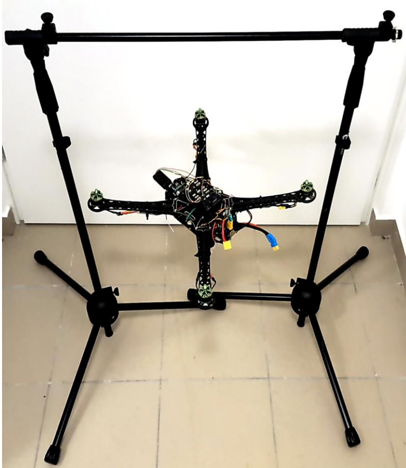
Figure 9. Photograph of the UAV inertia measurement setup.
