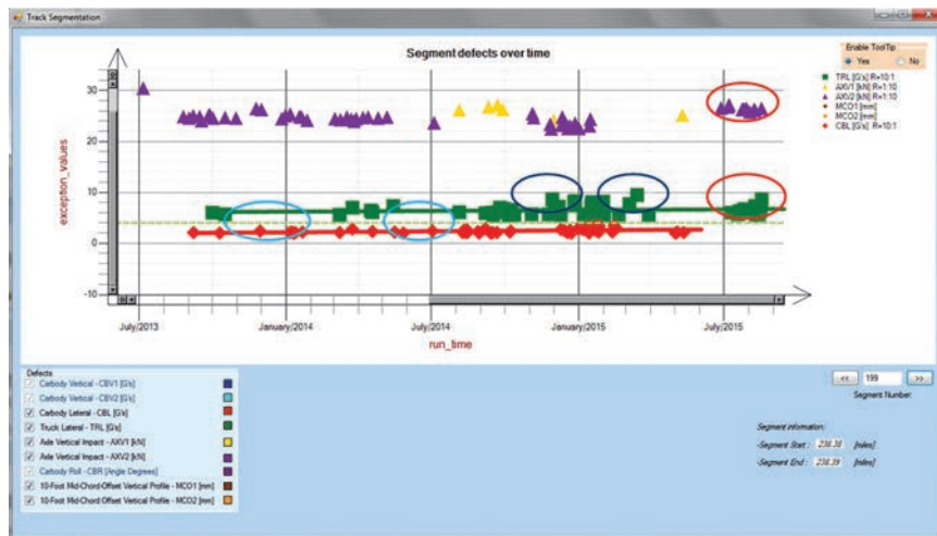
Figure 13 Connection between CBL and TRL defects [1]
