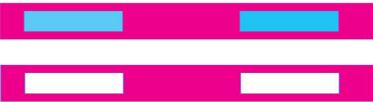
Figure 4. Test sample of the crispening effect with the secondary stimulus of 100% RTV and the primary stimuli of 55% RTV (left) and 65% RTV (right)
