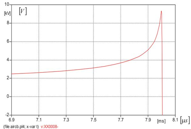
Fig. 3. Arc voltage in the air-blast circuit breaker
