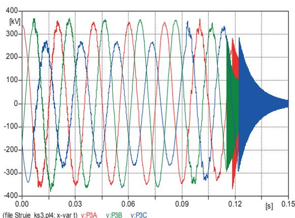
Fig. 8. Voltages on 400 kV side of transformer
