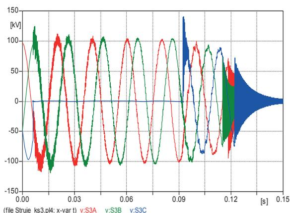
Fig. 7. Voltages on 110 kV side of transformer
