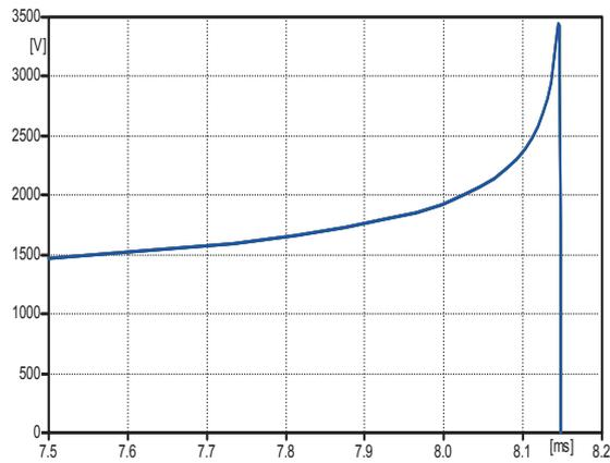
Fig. 2. Arc voltage in the SF<sub>6</sub> circuit breaker
