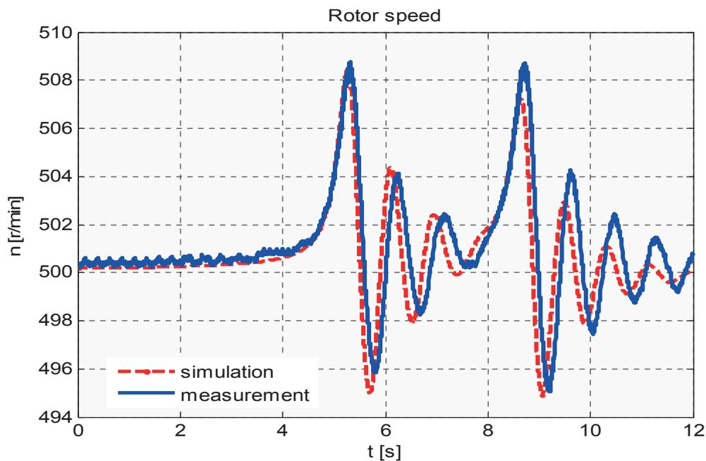
Figure 5 - Measured and simulated rotor speed
