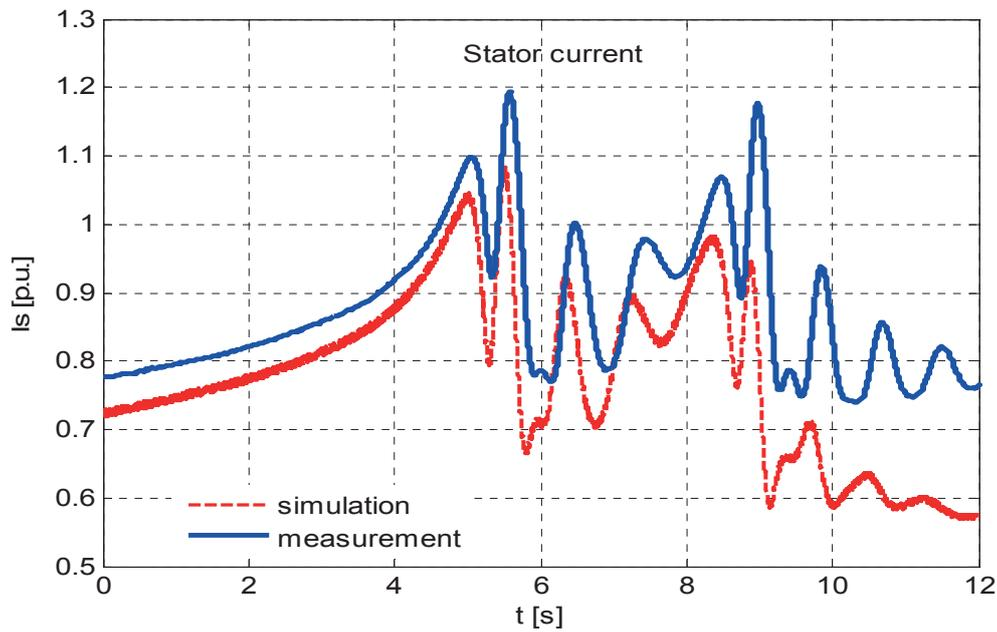
Figure 4 - Measured and simulated armature current
