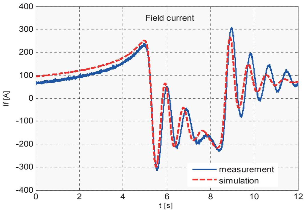
Figure 2 - Measured and simulated field current
