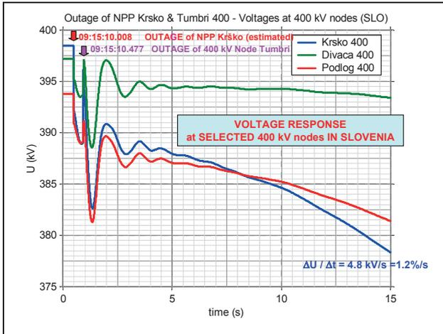
**Figure 13** Voltage at characteristic nodes of Slovenian system (outage of NPP Krško and 400 kV node Tumbri)
