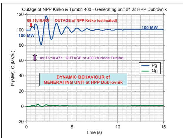
**Figure 15** Dynamic behavior of a generating unit of HPP Dubrovnik (outage of NPP Krško and 400 kV node Tumbri)
