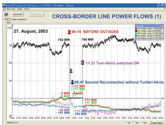
**Figure 5** Active power flows on lines between HR, SLO and H
