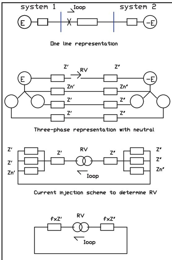
Fig. 3 Out-of-phase RV with  $f = \text{total } fpcf$
