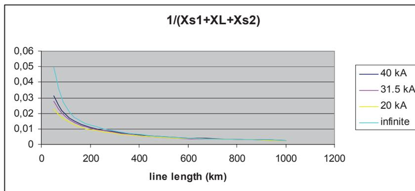
Fig. 6 Total admittance as function of line length
