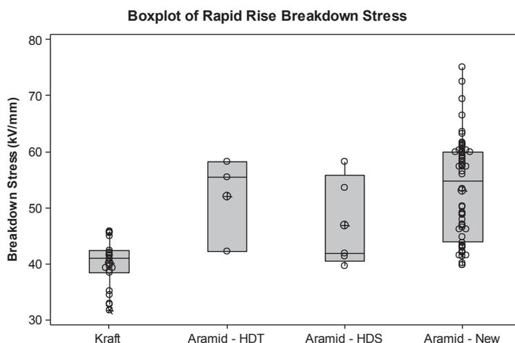
Figure 6 – Box Plot Comparing Rapid Rise Breakdown
