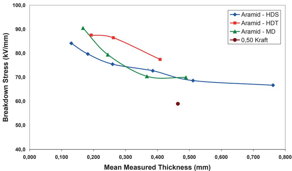
Figure 1 – Layer Insulation Breakdown Stress vs. Thickness
