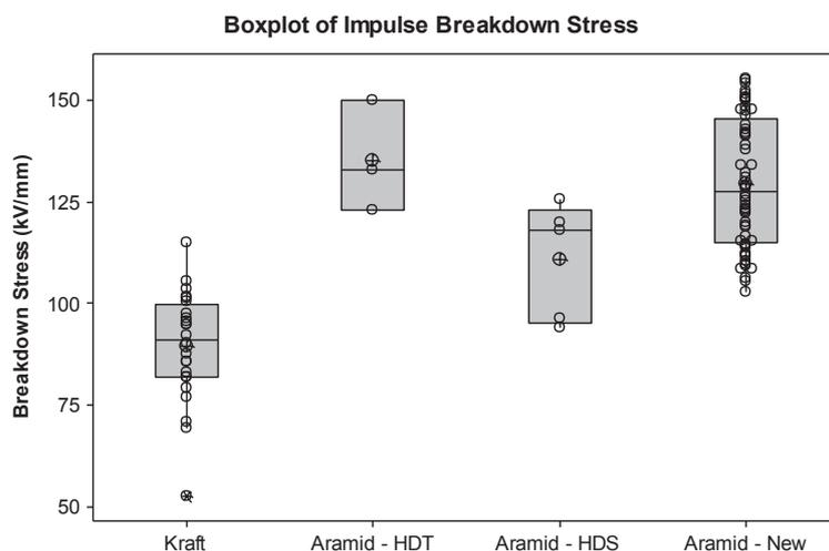
Figure 7 – Box Plot Comparing Impulse Breakdown
