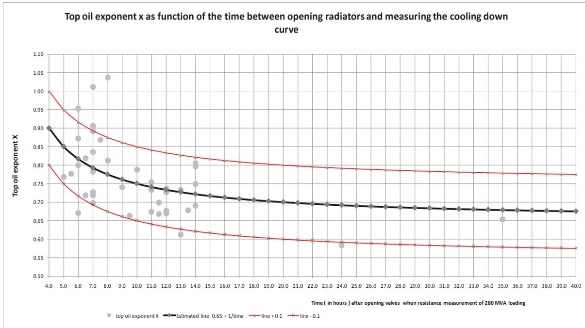
Figure 1 Top oil exponent x as function of time of switch off after opening cooler valves
