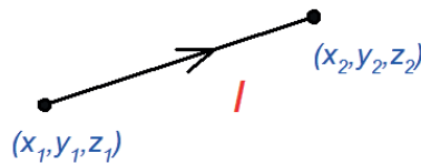
Figure 5 - A straight wire segment carrying current I
