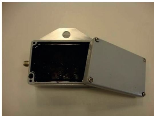
Figure 15 – Measuring impedance components sealed with water repellent compound
