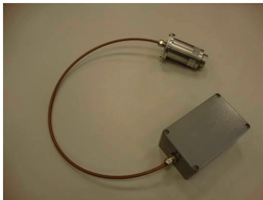
Figure 14 – Adapter and the measuring impedance
