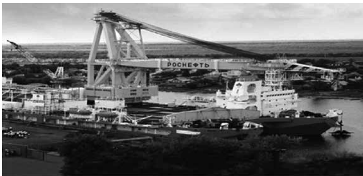
Figure 7 Catamaran crane of 12000 kN lifting capacity
