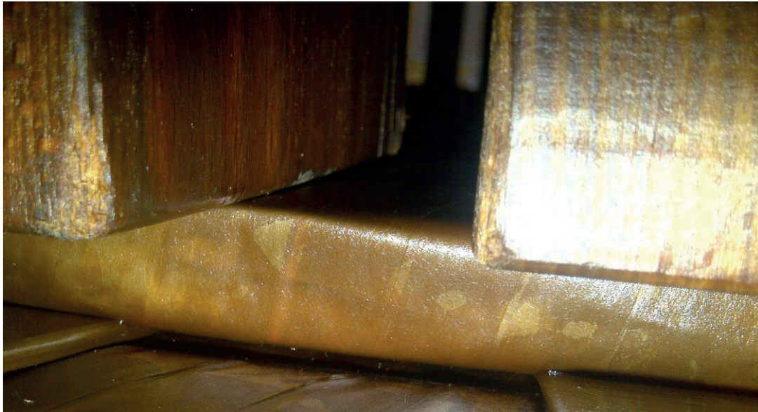
Figure 11 –Model 3 under the influence of the 100% of the critical tilting pressing force according to IEC
