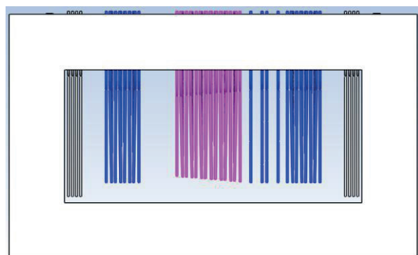
Figure 10: Short circuit condition being tested. Different colors represent opposing currents
