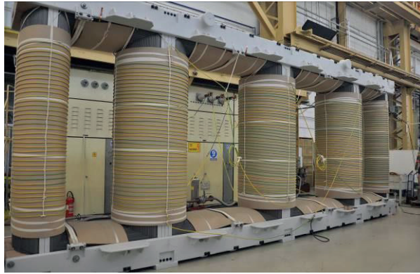
Figure 1 - Custom-made temporary windings during measurements
