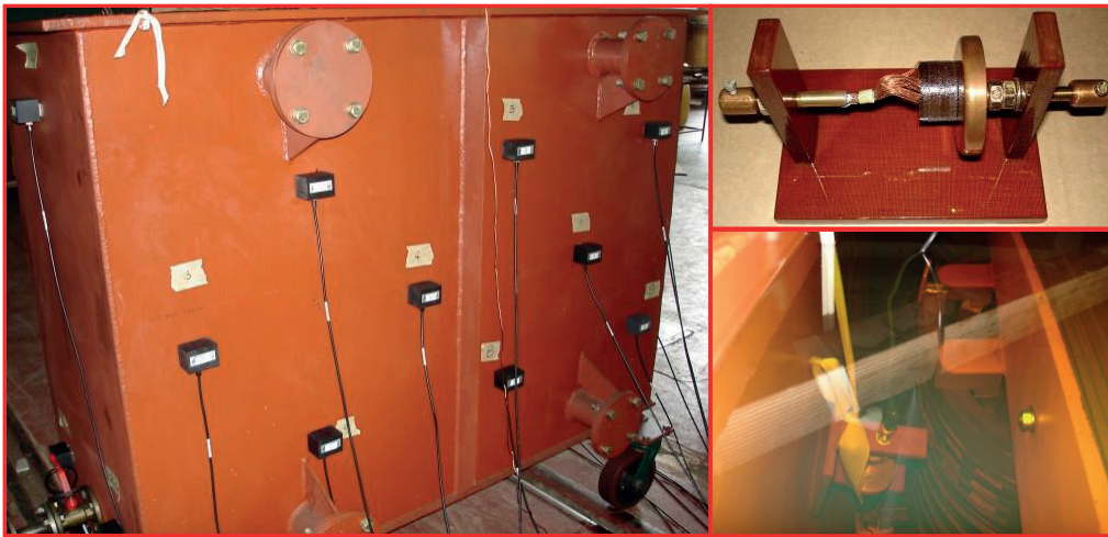
Figure 2. Sensor placement (left), PD source (right up) and its placement in the tank (right down).
