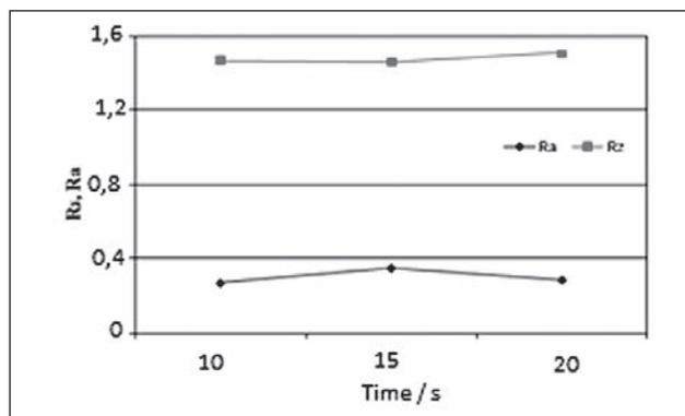
Figure 1 Relationship between roughness parameters of silver coatings  $R_a$  and  $R_z$  and application time (cathode current density 1 / A·dm<sup>-2</sup>)
