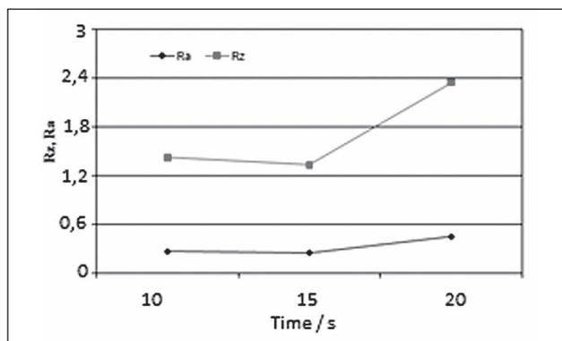
Figure 2 Relationship between roughness parameters of silver coatings  $R_a$  and  $R_z$  and application time (cathode current density 1,5 / A·dm<sup>-2</sup>, temp. 293 K)
