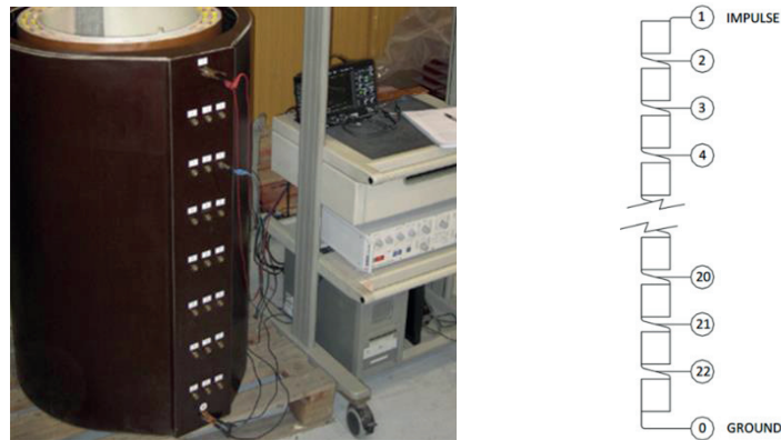
Figure 6 – Test arrangement (left) and HV measuring taps for the dry-type 1600 kVA transformer (right)
