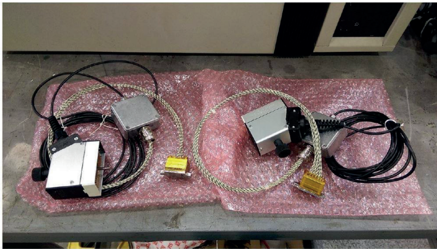
Figure 5: Two manufactured high temperature PA ultrasound probes using piezoelectric GaPO 4
