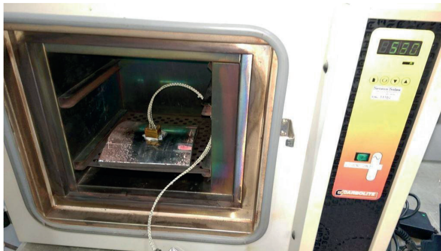
Figure 17: Phased array probe using GaPO 4 placed in an oven for characterisation at the target temperature of 580°C
