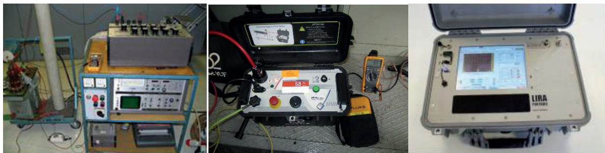
Figure 7: a) \tan \delta testing equipment with 50Hz and b) 0,1Hz and c) LIRA
