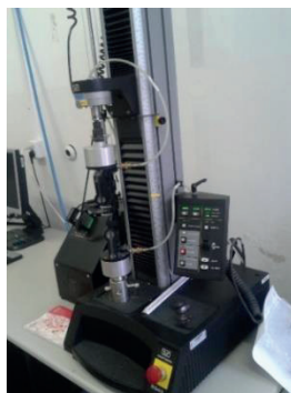
Figure 8: Testing equipment for EaB
