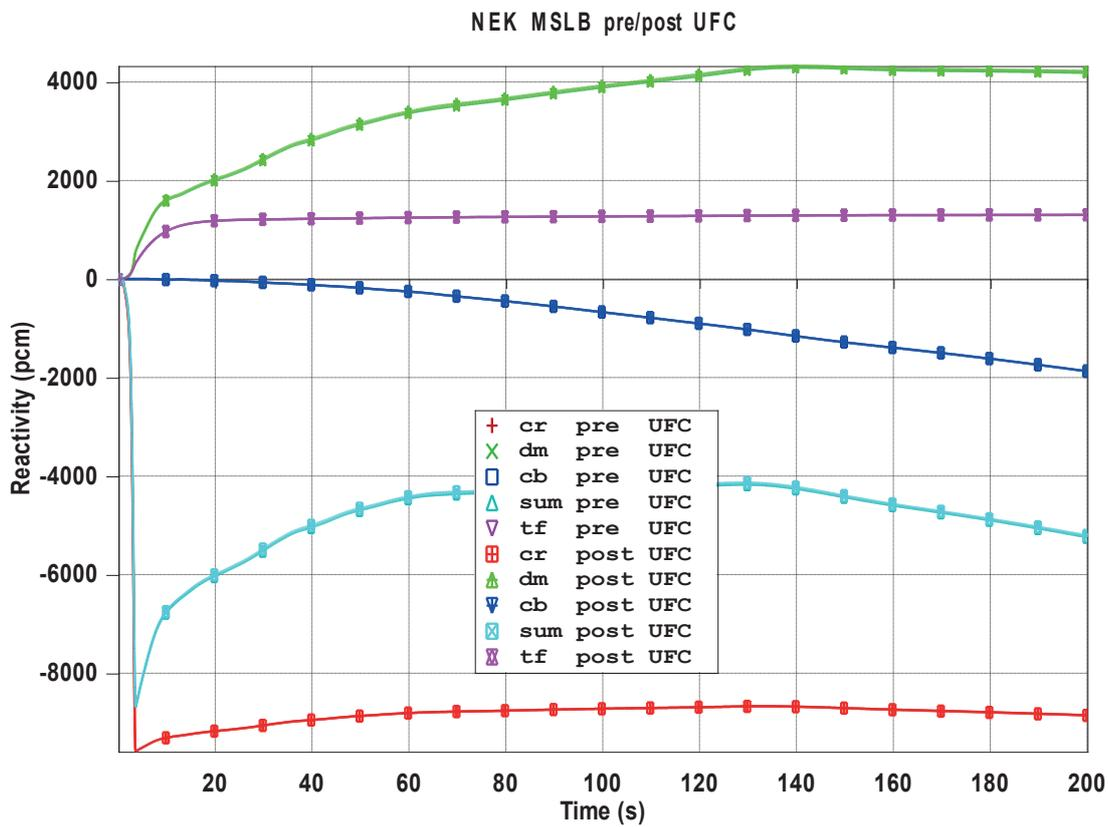
Figure 11: Reactivity components, pre vs. post UFC
