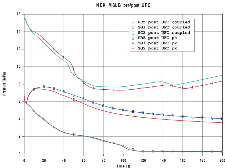
Figure 4: Pressurizer, Steam generator 1 and 2 pressure
