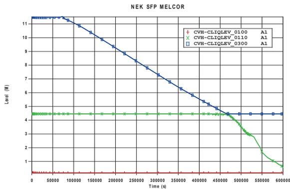
Fig. 4 Water elevation change in MELCOR
