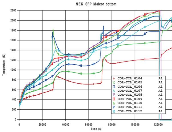
Fig. 10 Cladding temperature in Ring 1 (crack on bottom)
