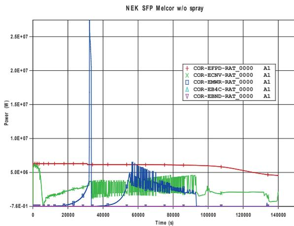
Fig. 11 Heat balance of pool contents - power
