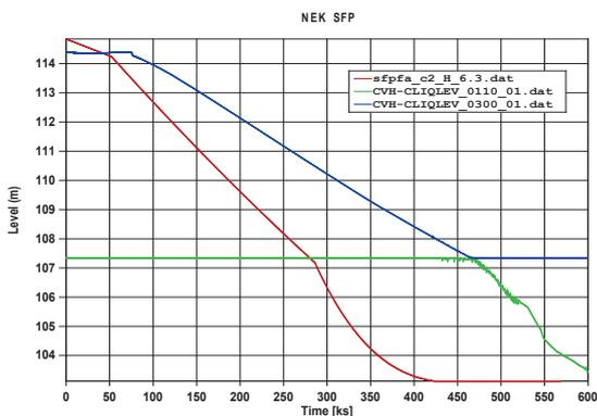
Fig. 5 MELCOR and SFPFA water elevation comparison
