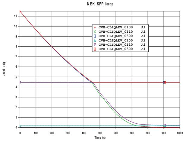
Fig. 8 Crack position impact on water level
