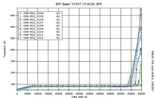
Fig. 7 Fuel cladding heatup in Ring 1
