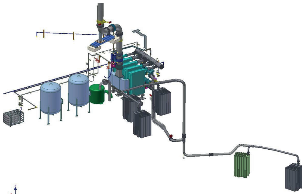
Figure 1. PCFV system layout, taken from [6]
