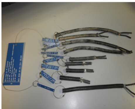
Fig. 4 Samples of 9 stages labelled oven aged cables with EPR insulation and CSPE jacket [9]
