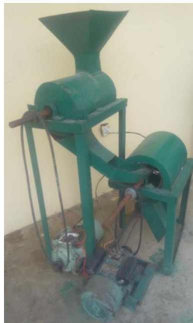
Fig. 2. Fabricated palm kernel cracking cum separation machine
