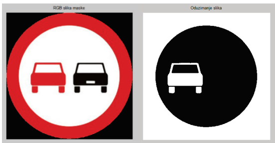
Figure 4 Mask of the RGB image and binary image obtained by subtraction of binary images
