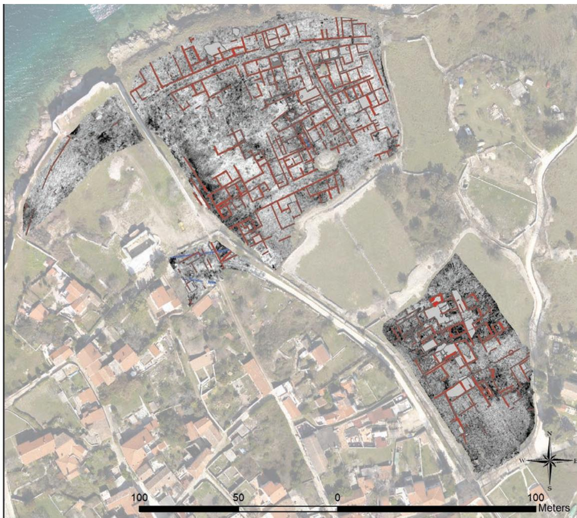
Fig. 12: Radargram and a general interpretation of the GPR data: walls (red), floors (gray) and water/power supply lines (blue). ©LBI ArchPro
