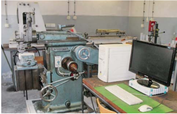
Figure 1: Linear cutting machine with measuring system with force transducer (Korman, 2014)
