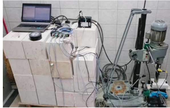
Figure 2: Laboratory drilling rig with measuring system for drilling energy measurement
