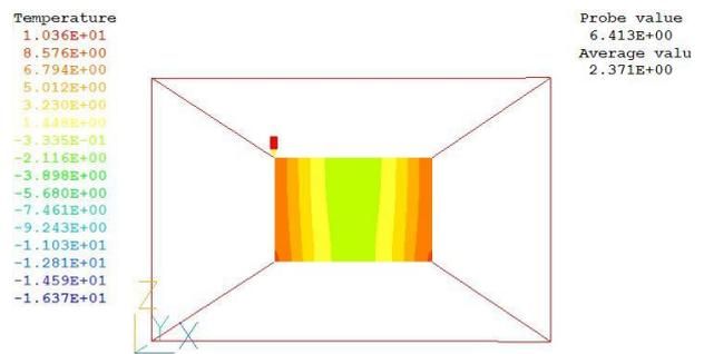
Figure 6. The temperature field of upper surface for heating layer while air velocity is 3.5m/s.
