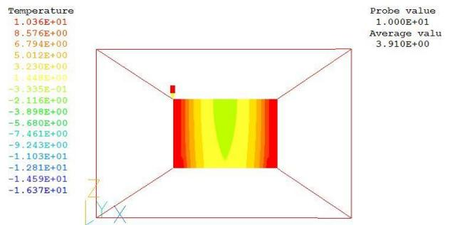
Figure 7. The temperature field of middle surface for heating layer while air velocity is 3.5m/s.
