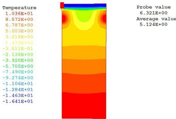
Figure 4. The temperature field of XY section of refrigerated warehouse floor while air velocity is 2.5m/s.
