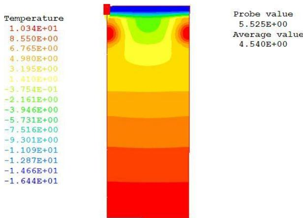
Figure 3. The temperature field of XY section of refrigerated warehouse floor while air velocity is 1.5m/s.
