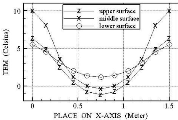
Figure 10. The temperature curves of points on upper, middle, and lower surface for heating layer while air velocity is 2.5m/s.
