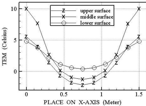
Figure 9. The temperature curves of points on upper, middle, and lower surface for heating layer while air velocity is 1.5m/s.
