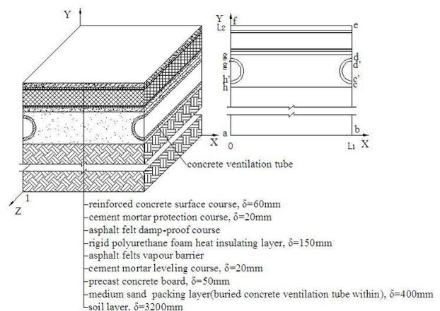
Figure 2. The calculating element of heat-transfer model for refrigerated warehouse floor.
