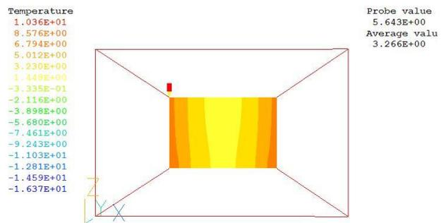
Figure 8. The temperature field of lower surface for heating layer while air velocity is 3.5m/s.
