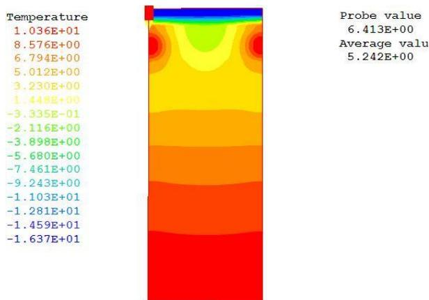
Figure 5. The temperature field of XY section of refrigerated warehouse floor while air velocity is 3.5m/s.
