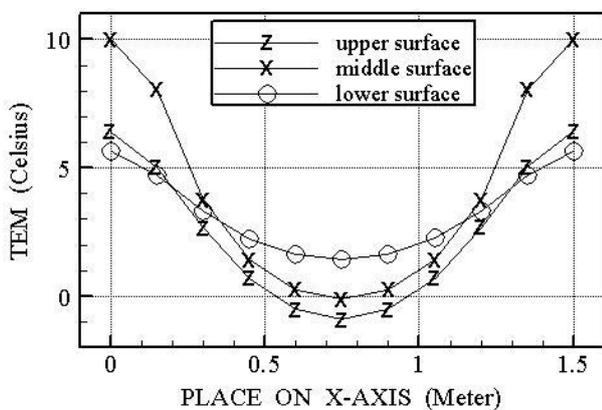
Figure 11. The temperature curves of points on upper, middle, and lower surface for heating layer while air velocity is 3.5m/s.
