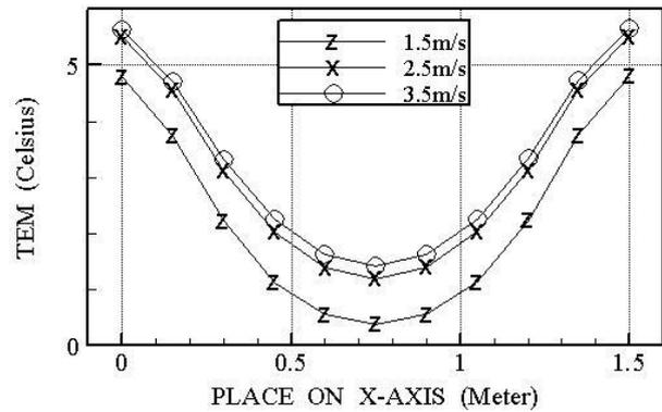
Figure 12. The temperature curves of points on lower surface for heating layer while air velocity is 1.5m/s, 2.5m/s and 3.5m/s.
