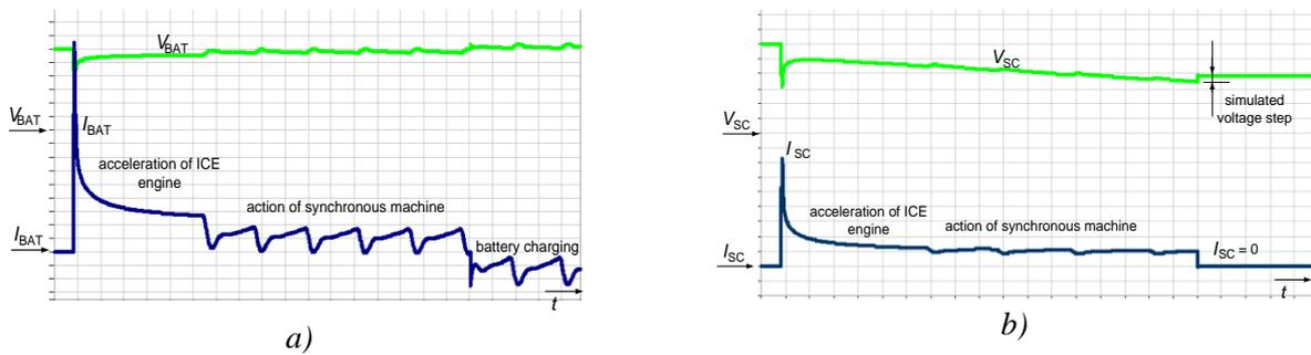
Figure 5. Simulated waveforms of DC bus voltage and current of the energy storage system during cranking; a) lead-acid battery successful cranking, b) supercapacitor unsuccessful cranking (25 A/div., 2 V/div., 100 ms/div.).
