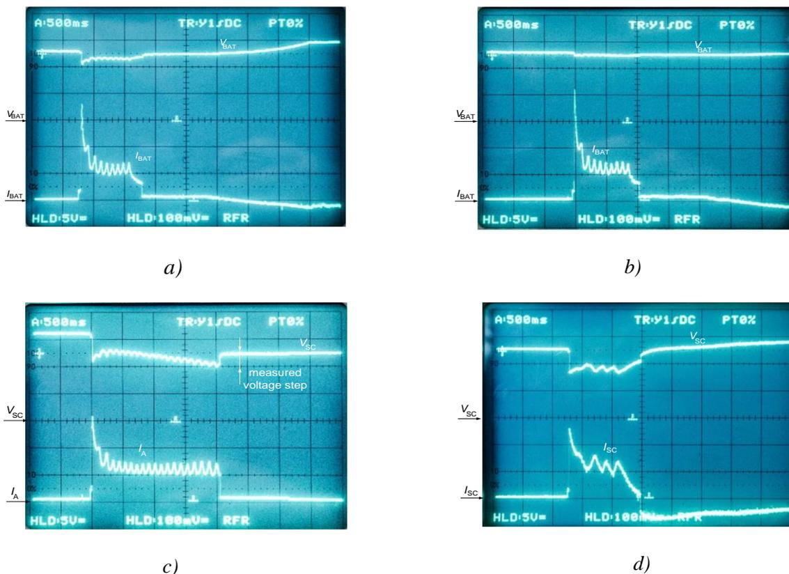
Figure 6. Measured waveforms of DC bus voltage and current of the energy storage system during cranking; a) lead-acid battery cranking, b) lead-acid battery with Li-ion battery and electrolytic capacitor cranking, c) supercapacitors unsuccessful cranking, d) successful cranking with supercapacitors (100 A/div., 5 V/div., 500 ms/div.).
