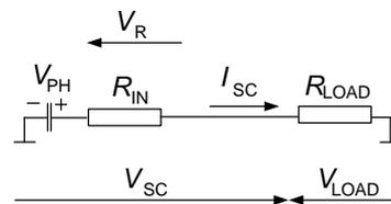
Figure 3. Simplified schematic of supercapacitor connected to the load.
