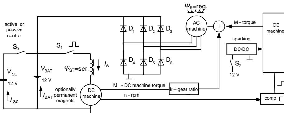
Figure 4. Simplified schematic of conventional car which enables simulation of different energy storage systems during cranking.
