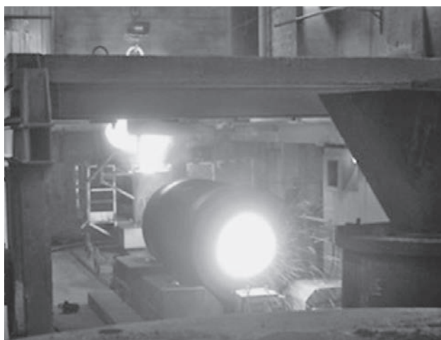
Figure 2 Centrifugal casting of the working shell
